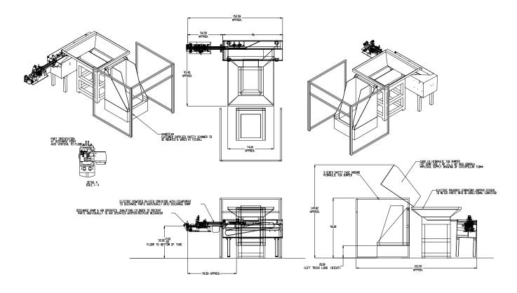
**APPLICATION:** Feed from a random loaded, floor mounted hopper. The Steel Tubular Slugs will be elevated
