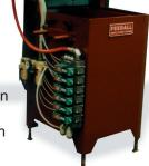
Parts fed: .375" dia. x 3.500" to 8.000" lg. @ 40 per min.
