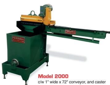
base for feeding a centerless grinder. Parts fed: 1/4" to 1/2" dia. x .700 to 8" lg. @ 200" per min.
