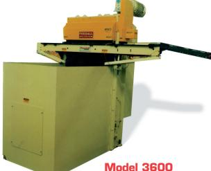
c/w 1" wide x 84" conveyor, and roller chute. Feeding an end facing machine. Parts fed: .800" to 1.100" dia. x 2.600" to 3.44" lg. @ 75 to 100 per min.
