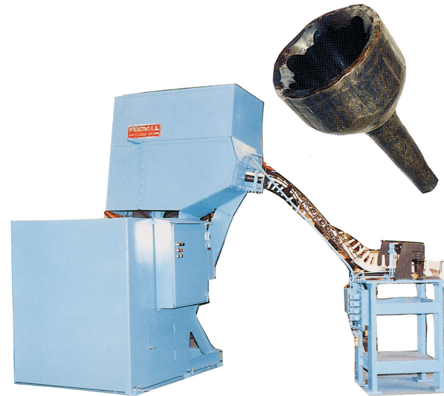
Model 2500-HD c/w two position robot pickup station. Parts fed and oriented: automotive front wheel drive spindle forgings, feeding a dual spindle CNC lathe via loader robot.
