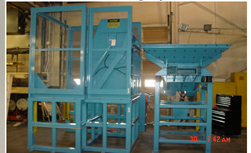
Dumper w/Vibratory Metering Hopper
