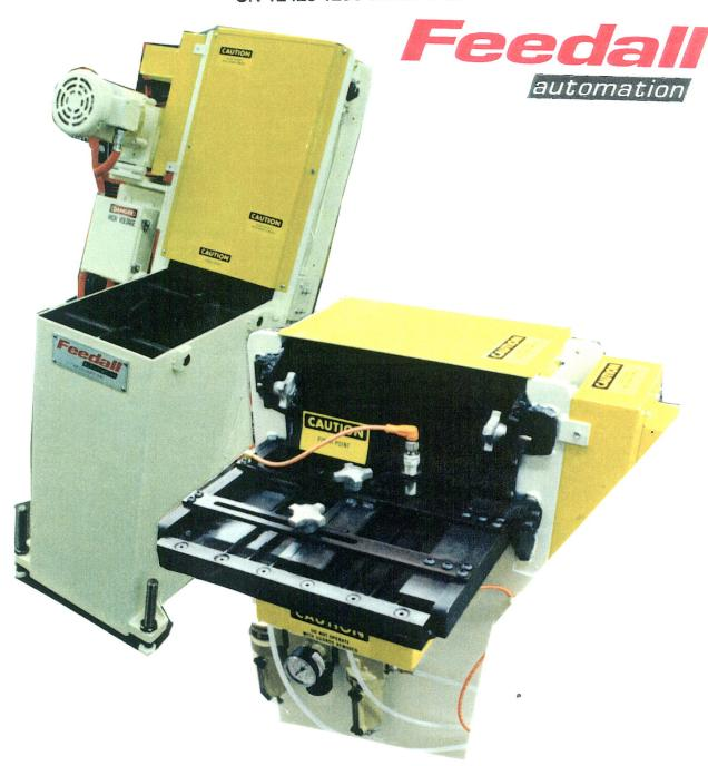
FEED FROM A MANUALLY STACKED HOPPER, DC ARMATURE SHAFTS .370 TO .400 DIA. X 4 1/2 TO 7" LG. THE SHAFTS ARE ESCAPED ROLLING ONE AT A TIME FROM THE REAR OF THE ELEVATOR AT A HEIGHT OF 42 1/2" AT A RATE OF 40 PER. MIN.
