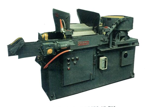
FEED FROM A MANUALLY LOADED MAGAZINE RODS, 3/8, 7/16, 1/2, 5/8, AND 3/4" DIA. X 3 1/2 TO 12" LG. IN A FEEDER BOWL RODS, SAME DIAS. X 1 TO 3 1/4" LG. RODS WILL BE FED TO THE FRONT MOUNTED CROSS CONVEYOR THEN CONVEYED END TO END TO A CENTERLESS GRINDER AT 42" ABOVE THE FLOOR AT A RATE OF 120" PER. MIN. DWG. P 7636
