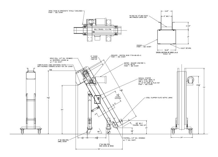
**APPLICATION:** Convey Universal Joint Bearing Cups from 15" to 60" above the floor.
