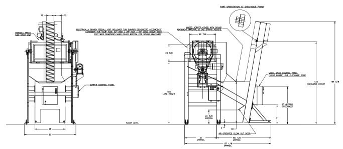
**APPLICATION:** Feed from a random loaded, floor mounted hopper. The blanks will be elevated from the
