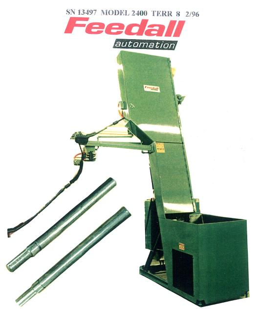
FEED FROM A RANDOM LOADED FLOOR HOPPER ARMATURE SHAFTS 1/2" DIA. BY 63/8" LG. THE SHAFTS WILL BE ELEVATED AND FED END TO END TO ORIENTER, THEN ORIENTED SMALL DIA. LEADING AND FED END TO END TO A CENTERLESS GRINDER AT 42" ABOVE THE FLOOR AT A FEED RATE OF 20 PARTS PER. MIN. DWG P 9105 R3
