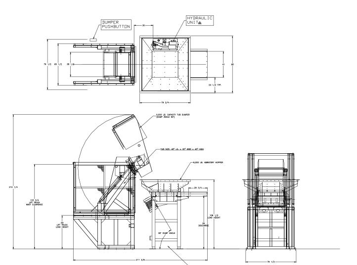
**APPLICATION:** Feed from a random loaded floor mounted hopper. These parts will be dumped from a tub
