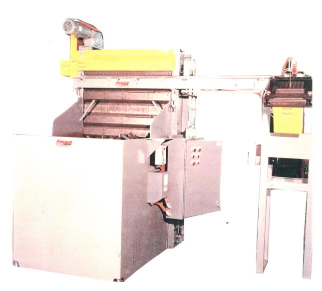
FEED FROM A RANDOM LOADED FLOOR MOUNTED HOPPER SHEAR CUT STEEL BILLETS 1 9/32 TO 1 3/4 DIA.X 10 TO 15" LG. THE BILLETS WILL BE ELEVATED FROM THE HOPPER THEN DISCHARGED ROLLING TO THE FRONT MOUNTED CROSS CONVEYOR THEN FED END TO END TO A TRANSFER DEVICE THEN TRANSFERRED ROLLING INTO A SINGLE ROW MAGAZINE AND ESCAPED ONE AT A TIME ON SIGNAL TO A WALKING BEAM AT 71" ABOVE THE FLOOR AT A RATE OF 300 TO 500 BILLETS PER. HOUR. 48" WIDE ELEVATOR BELT, 30 CU. FT. HOPPER
