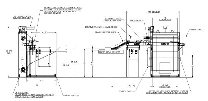
**APPLICATION:** Feed from a random loaded, floor mounted hopper. The Steel Billets will be elevated from the
