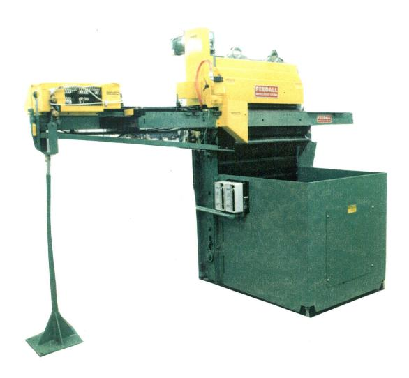
FEED FROM A RANDOM LOADED FLOOR MOUNTED HOPPER THREADED STUDS 1/2,5/8,3/4,7/8 AND 1" DIA. X 2 TO 10" LG. THE STUDS WILL BE ELEVATED FROM THE HOPPER THEN DISCHARDED ROLLONG TO THE FRONT CROSS CONVEYER THEN FED END TO END TO A TRANSFER DEVICE THEN TRANSFERRED ROLLING AT A HEIGHT OF 54" ABOVE THE FLOOR TO A NUT INSTALLER AT A RATE OF 60 PER. MIN. 36" WIDE ELEVATOR, 12 CU. FT. HOPPER
