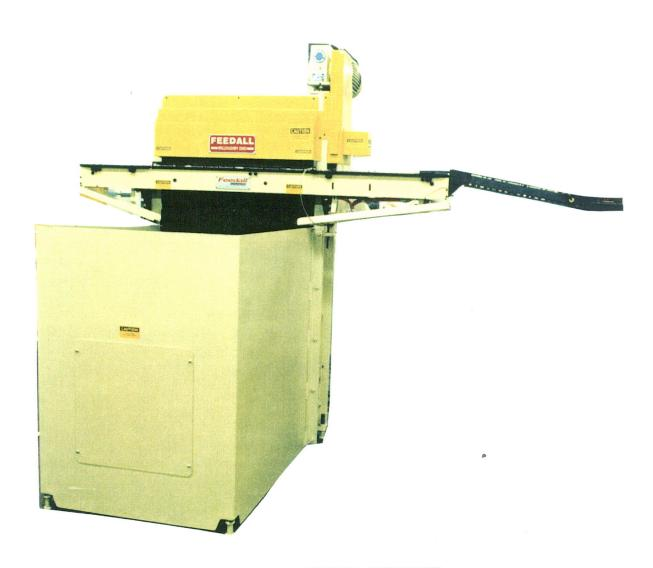
FEED FROM A RANDOM LOADED FLOOR MOUNTED HOPPER AUTOMOTIVE PISTON PINS . 825 TO 1.054 "DIA.X 2.62 TO 3.44" LG. THE PINS WILL BE ELEVATED FROM THE HOPPER THEN DISCHARGED ROLLING TO THE FRONT CROSS CONVEYOR THEN FED END TO END TO AN ECONOMY END FINISHER. THE FEED RATE WAS 4500 PINS PER. HOUR.
