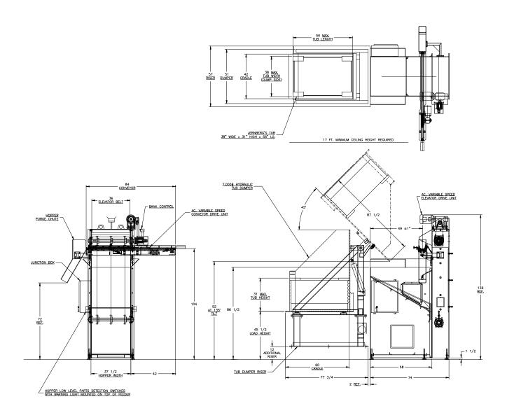
**APPLICATION:** Feed from a random loaded, floor mounted hopper. The Saw-Cut and Sheared Billets will be
