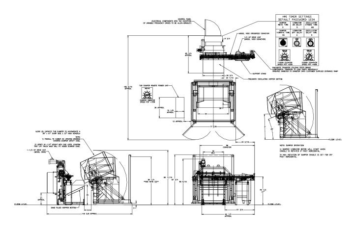
**APPLICATION:** Feed from a random loaded, floor mounted hopper. The track pins will be metered from a tub
