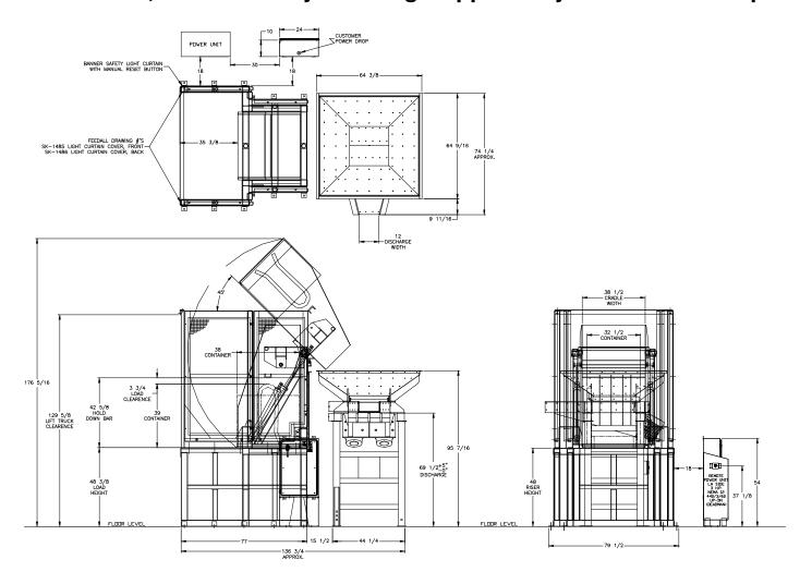
**APPLICATION:** Feed from a manually loaded, floor mounted hopper, then metered into a Vibratory Bowl Feeder
