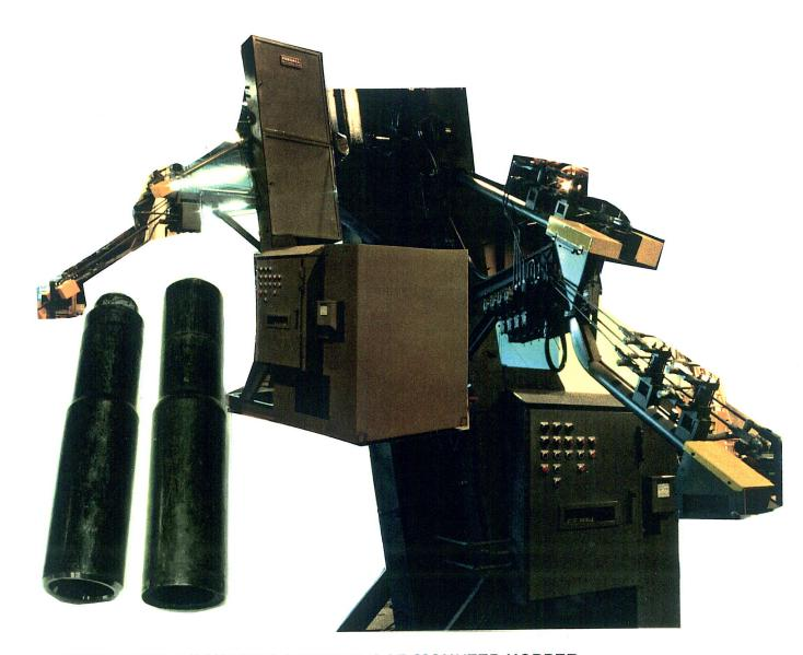
FEED FROM A RANDOM LOADED FLOOR MOUNTED HOPPER, AUTO BUMPER ISOLATOR TUBE EXTRUSIONS, 1 1/2" DIA. X 10" LG. THE TUBES WILL BE ORIENTED END TO END SLIDING, THEN ORIENTED CLOSED END LEADING AND THEN TRANSFERRED ROLLING AT A HEIGHT OF 50" ABOVE THE FLOOR AT A RATE OF 1500 PER HOUR TO A DOUBLE END FACING MACHINE.
