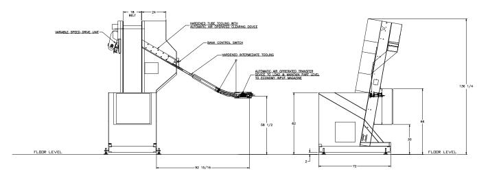
**APPLICATION:** Feed from a random loaded, floor mounted hopper. The Steel Tubes will be elevated from
