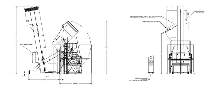
**APPLICATION:** Feed from a random loaded, floor mounted hopper. The blanks will be elevated from the
