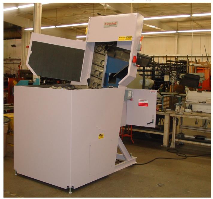
**APPLICATION:** Feed from a random loaded, floor mounted hopper, Tapered Roller Bearing Cup Forgings. Forgings are elevated out of hopper with cleated belt and discharged in a continuous.
