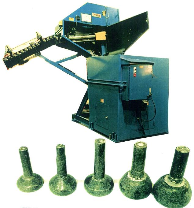
FEED FROM A RANDOM LOADED FLOOR HOPPER, ELEVEN VARIOUS SIZE OUTER RACE EXTRUSIONS. THE RACES ARE ELEVATED FROM THE HOPPER THEN DISCHARGED SLIDING OVER DRIVEN FEED ROLLS AND ORIENTED HEAD UP AXIS VERTICAL THEN FED DIAMETER TO DIAMETER THROUGH A SLIDING CHUTE TO THE INPUT CHUTE OF A BLISS PRESS AT 62" ABOVE THE FLOOR AT A FEED RATE OF 25 PER. MIN.
