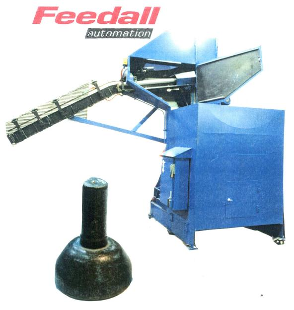
FEED FROM A RANDOM LOADED FLOOR MOUNTED HOPPER, AUTO CV JOINT OUTER RACES. THE RACES ARE ORIENTED HEAD UP, AXIS VERTICAL AND FED IN A SINGLE STREAM TO A PRESS AT A HEIGHT OF 52" ABOVE THE FLOOR AT A FEED RATE OF 25 PER. MIN. 12" WIDE ELEVATOR, 30 CU. FT. HOPPER DWG. PD 8922 R 2
