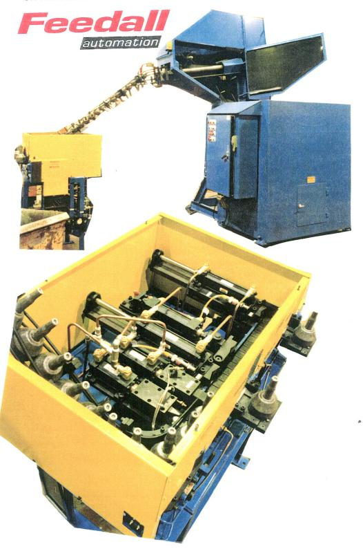
FEED FROM A RANDOM LOADED FLOOR MOUNTED HOPPER, AUTO CV JOINT OUTER RACES. THE RACES ARE TO BE ORIENTED STEM UP IN AN AXIS VERTICAL POSITION IN TWO INDEPENDENTLY CONTROLLED STREAMS, THEN POSITIONED ON DEMAND TO ONE OR TWO ROBOT PICK UP POINTS LOCATED 18" APART AND 45".
