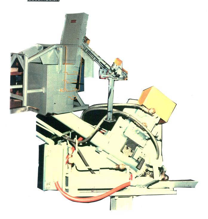
FEED FROM A RANDOM LOADED FLOOR MOUNTED HOPPER SHEARED STEEL BILLETS, 1.937 TO 2.625" DIA. X 2.00 TO 3.25" LG. THE BILLETS WILL BE ORIENTED IN TO A SINGLE END TO END STREAM, THEN TRANSFERRED ONE AT A TIME ROLLING IN TO A PUSHER DEVICE, WHICH WILL ADVANCE EACH BILLET TO AN INDUCTION COIL AT 60" ABOVE THE FLOOR AT A RATE OF 350 TO 450 PER. HOUR FOR FORGING. 12" WIDE ELEVATOR BELT, 30 CU. FT. HOPPER. DWG PD 7152
