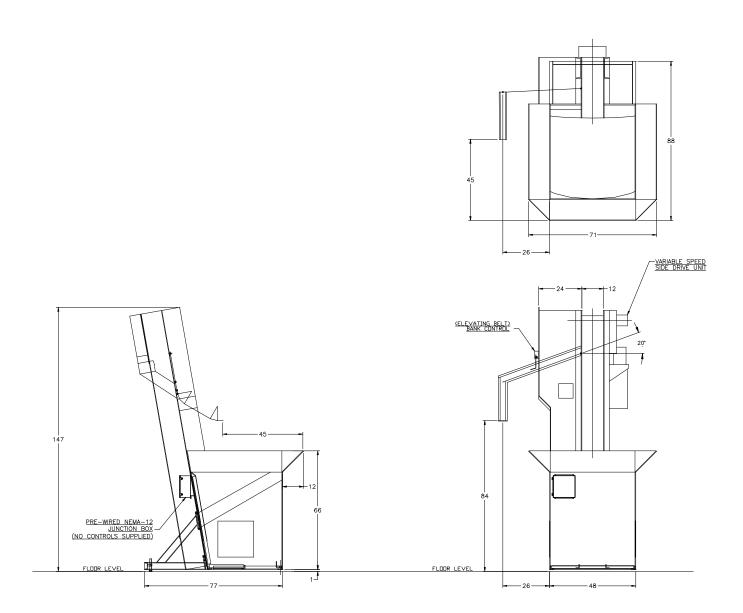
**APPLICATION:** Feed from a random loaded, floor mounted hopper. The Saw Cut Steel Slugs will be elevated
