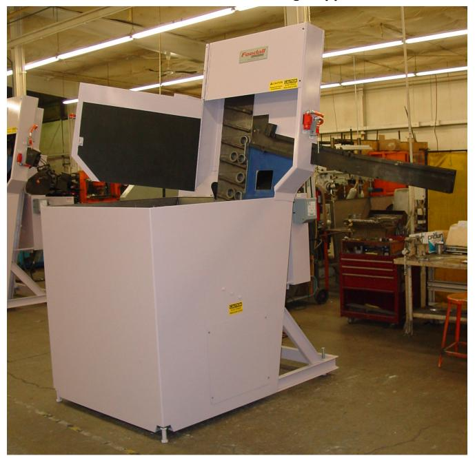
**APPLICATION:** Feed from a random loaded, floor mounted hopper, Tapered Roller Bearing Cone Forgings.
