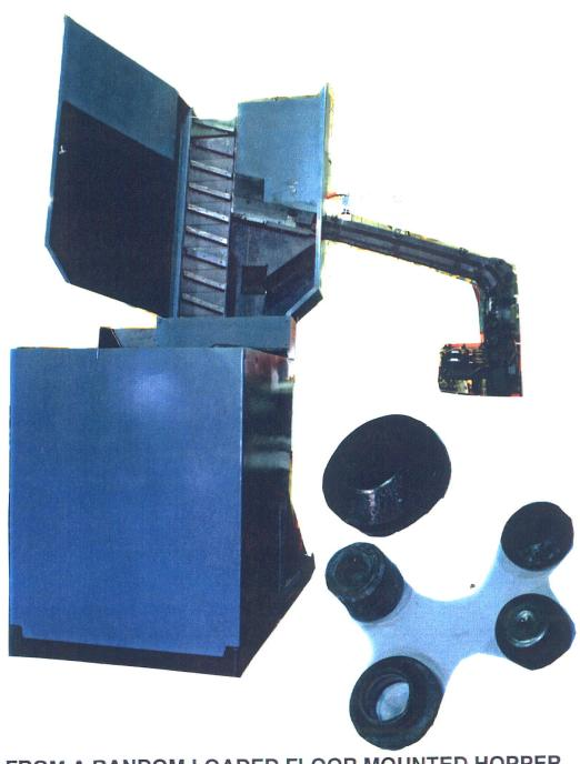
FEED FROM A RANDOM LOADED FLOOR MOUNTED HOPPER, ASSORTED PREFORMS TO BE ORIENTED DIAMETER TO DIAMETER ROLLING THEN ESCAPED ONE AT A TIME LAYING FLAT TO A CONVEYOR AT 55" ABOVE THE FLOOR AT A RATE OF 55 PER. MIN. FOR A BILLET WEIGHT SEGREGATOR. 12" WIDE ELEVATOR BELT, 20 CU. FT. HOPPER. DWG. P 8939
