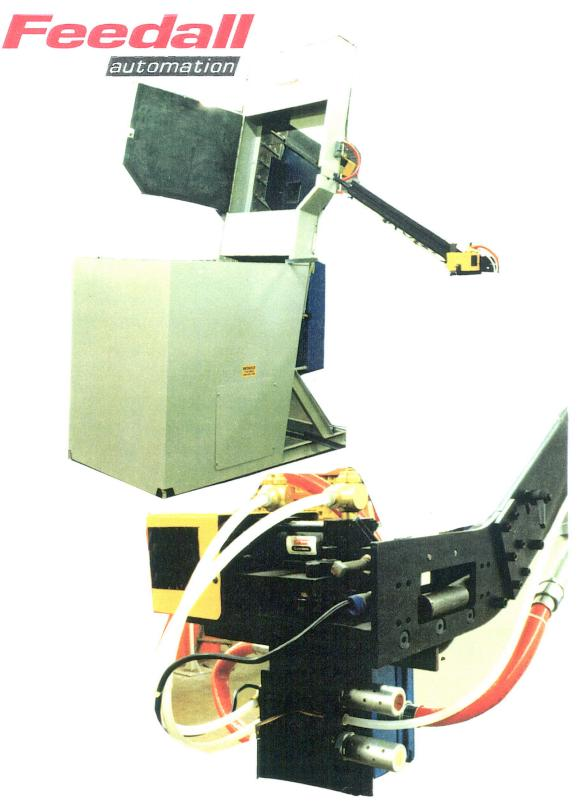
FEED FROM A RANDOM LOADED FLOOR MOUNTED HOPPER, PISTON WRIST PINS .75 TO 1.50" DIA. X 2 TOP 4 LG. THE PINS ARE TO BE ORIENTED AND FED IN A SINGLE ROLLING DIAMETER TO DIAMETER STREAM TO THE INPUT OF THE ECONOMY END FINISHER MAGAZINE AT A HEIGHT OF 59" ABOVE THE FLOOR AT A FEED RATE OF 40 TO 60 PARTS PER. MIN.
