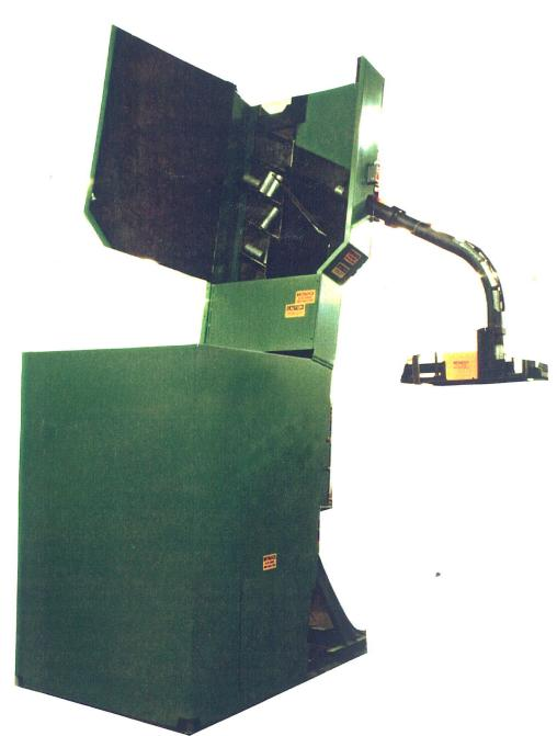
FEED FROM A RANDOM LOADED FLOOR MOUNTED HOPPER, SAW CUT BILLETS, 2 1/2 TO 3" DIA. X 5 TO 6" LG. THE BILLETS WILL BE ORIENTED END TO END AND FED INTO A VERTICAL CHUTE, THEN TRANSFERRED DIAMETER TO DIAMETER ONE AT A TIME AT A HEIGHT OF 60" ABOVE THE FLOOR AT A RATE OF 6 TO 10 PER. MIN. TO A PRESS.
