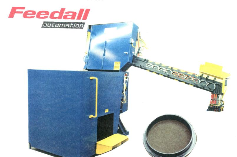
FEED FROM A RANDOM FLOOR MOUNTED HOPPER, OUTER BEARING CAGES 2.515 TO 4.615" DIA. X .508 TO .725" WIDE. THE CAGES ARE ORIENTED AND DELIVERED LAYING FLAT, FLANGE DOWN ON CUSTOMERS CONVEYOR AT A RATE OF 20 PER. MIN. AT 36" ABOVE THE FLOOR.
