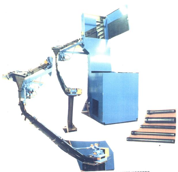
FEED FROM RANDOM LOADED FLOOR MOUNTED HOPPERS EXTRUDED METAL HYDRAULIC HOSE STEMS, .502 TO .972 "DIA. X 4.252 TO 7.913" LG. (MODEL 2500D) AND 1.500 TO 3.125" DIA. X 4.310 TO 12.70" LG. (MODEL 2600HD) THE HOSE STEMS WILL BE ORIENTED WITH SMALL DIA. STEM AND LEADING AND TRANSFERRED ONE AT A TIME, AXIS HORIZONTAL, TO A LOAD NEST AT 45" ABOVE THE FLOOR AT A FEED RATE OF 150 TO 300 PER. HOUR.
