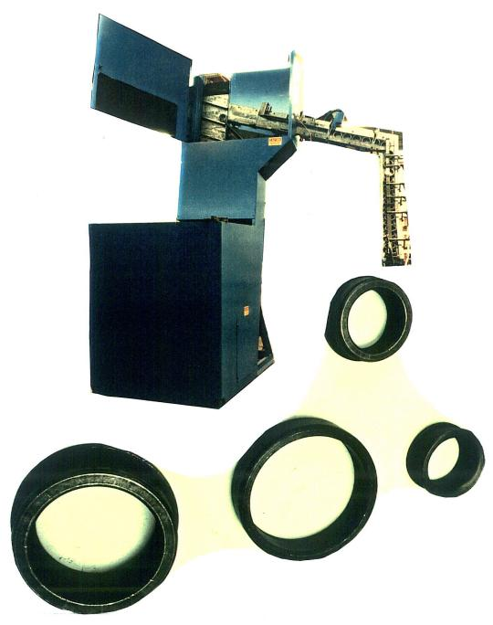
FEED FROM A RANDOM LOADED FLOOR MOUNTED HOPPER, INNER AND OUTER BEARING RACES 1.75 TO 5.0" DIA.X .57 TO 1.6" THICK. THE BEARINGS WILL BE ORIENTED DIAMETER TO DIAMETER ROLLING IN A SINGLE STREAM THEN FED TO A POSITION 48" ABOVE THE FLOOR LAYING FLAT AXIS HORIZONTAL TO THE CUSTOMERS CONVEYOR AT A RATE OF 20 TO 30 PER. MIN.
