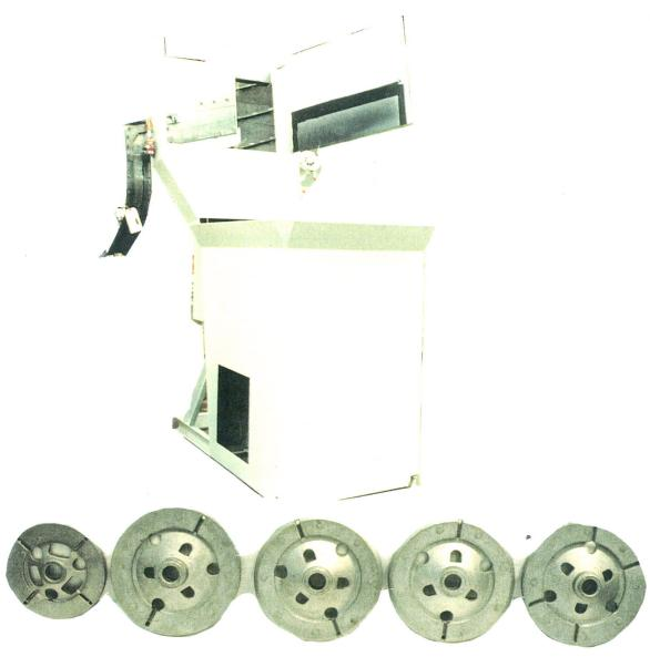
FEED FROM A RANDOM LOADED FLOOR MOUNTED HOPPER, ALUMINUM CAST CLUTCH DISCS, THE DISCS WILL BE ELEVATED FROM THE HOPPER THEN FACE ORIENTED AND FED DIAMETER TO DIAMETER HORIZONTAL HUB DOWN TO A POINT 48" ABOVE THE FLOOR AT RATE OF 720 PER. HOUR. TO A MACHINE CELL.
