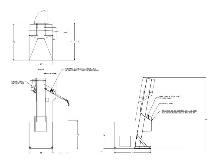
**APPLICATION:** Feed from a random loaded, floor mounted hopper. The Stampings will be elevated from the
