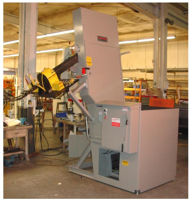
**APPLICATION:** Feed from a random loaded, floor mounted hopper, Engine Bulkhead Insert Forgings.
