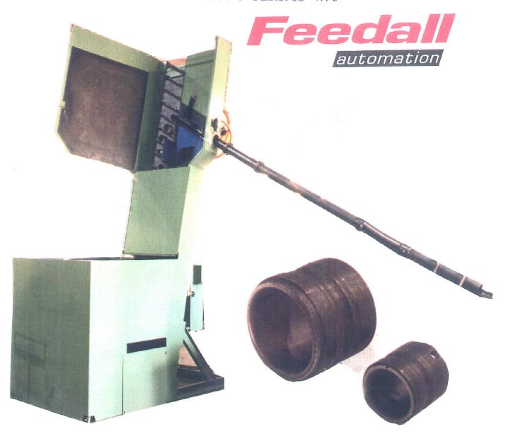
FEED FROM A RANDOM LOADED FLOOR HOPPER INNER BEARING RACES 1.50" TO 3.03" DIAMETER BY 1.40" TO 2.51" LONG. THE RACES WILL BE ORIENTED END TO END SLIDING IN A CONTINOUS STREAM AND FED TO A CENTERLESS GRINDER AT 42" ABOVE THE FLOOR AT A FEED RATE OF 700 TO 1500 PARTS PER. HOUR. 12" WIDE ELEVATOR BELT, 14 CUBIC FOOT HOPPER. DWG P 9178 R2
