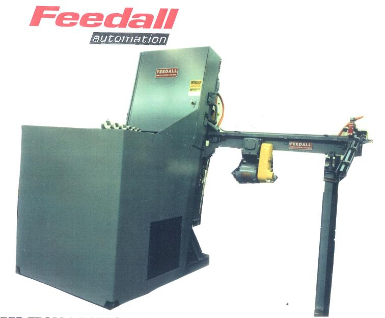
FEED FROM A RANDOM LOADED FLOOR HOPPER, COUPLINGS 1/2, 3/4, 1, 1 1/4, 1 1/2 & 2 NPT. PARTS ARE ELEVATED FROM THE HOPPER THEN ORIENTED END TO END AND FED TO A CONVEYOR THEN TRANSFERRED ROLLING ONE AT A TIME INTO A CHUTE TO AN AUTOMATIC ASSEMBLY MACHINE THAT THREADS ONE COUPLING ON A CONDUIT TUBE. AT A RATE OF 1500 TO 3000 PER. HOUR AT A HEIGHT OF 47" ABOVE THE FLOOR. DWG. P 7997. 12" WIDE ELEVATOR BELT, 14 CUBIC FOOT HOPPER, 62" LONG CONVEYOR AND PNEUMATIC TRANSFER.
