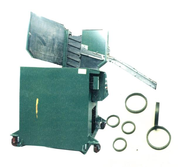
FEED FROM A RANDOM LOADED FLOOR MOUNTED HOPPER, VALVE SEAT INSERTS .987 TO 2.06" DIA. X .200 TO .400 " THICK. THE PARTS WILL BE ELEVATED FROM THE HOPPER THEN ORIENTED ROLLING DIAMETER TO DIAMETER IN A SINGLE STREAM FED TO A DOUBLE DISC.
