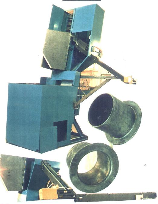
FEED FROM A RANDOM LOADED FLOOR HOPPER, STEEL DEEP DRAWN BUSHINGS 2 1/2" DIA. THE BUSHINGS ARE ELEVATED FROM THE HOPPER AND ORIENTED HANGING BY THE FLANGE THEN FED TO A PUSHER DEVICE AND ADVANCED ONE AT A TIME IN TO A HORIZONTAL CHUTE DIA. TO DIA. TO THE PRESS LOAD STATION AT 67" ABOVE THE FLOOR AT A RATE OF 30 TO 50 PER. MIN.
