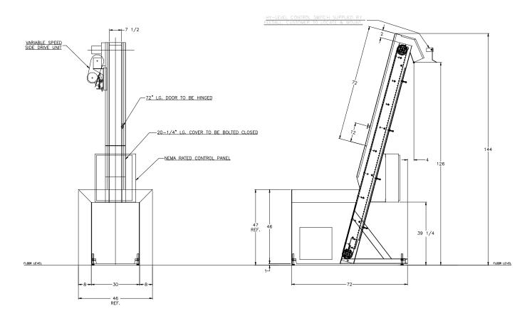
**APPLICATION:** Feed from a random loaded, floor mounted hopper. The parts will be elevated from the
