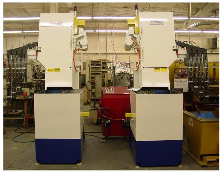
**APPLICATION:** Feed from a random loaded, floor mounted hopper, Universal Joint Bearing Cups. Cups will
