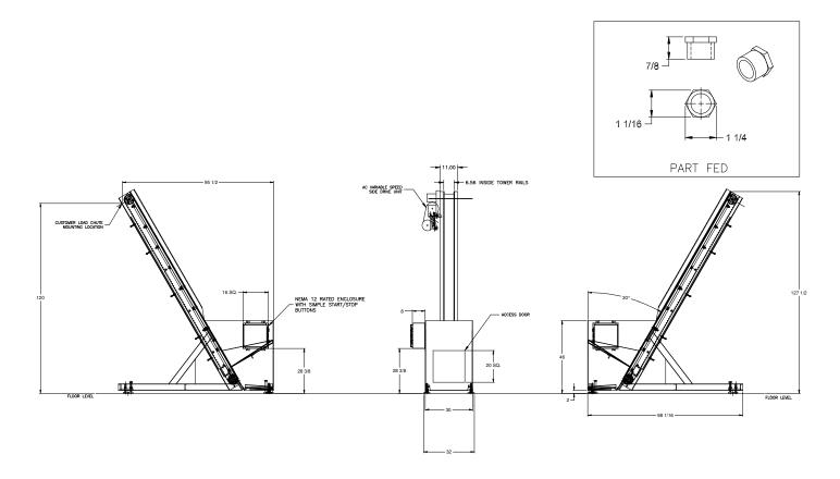
**APPLICATION:** Feed from a random loaded, floor mounted hopper. Hex Head Fasteners will be elevated
