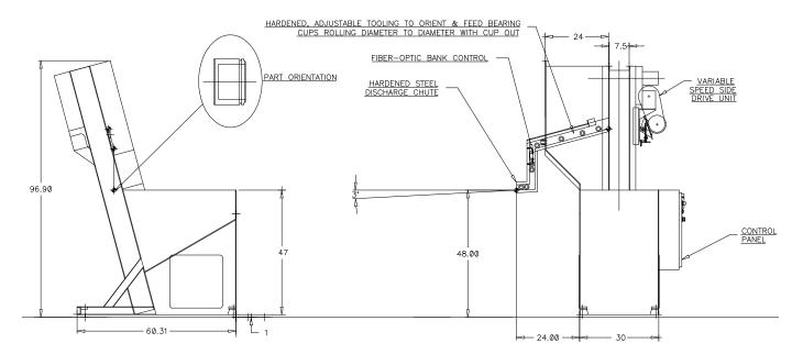
**APPLICATION:** Feed from a random loaded, floor mounted hopper. The Bearing Cups are coated with rust
