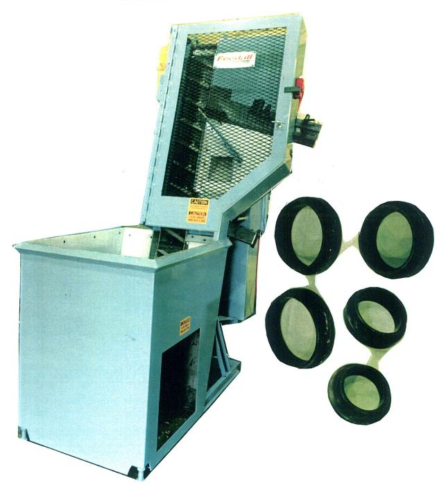
FEED FROM A RANDOM LOADED FLOOR HOPPER INNER BEARING RACES 1.250" TO 2.75" DIA. BY .375" TO .750" THICK. THE RACES ARE ELEVATED FROM THE HOPPER THEN DISCHARGED ROLLING THROUGH ORIENTING TOOLING, FACE ORIENTED THEN FED DIA. TO DIA. ROLLING TO A BALL RACE GRINDER AT 66" ABOVE THE FLOOR AT A RATE OF 1200 PER. HR. 7 1/2" WIDE ELEVATOR BELT, 8 CUBIC FOOT HOPPER. DWG. P9434 R 2
