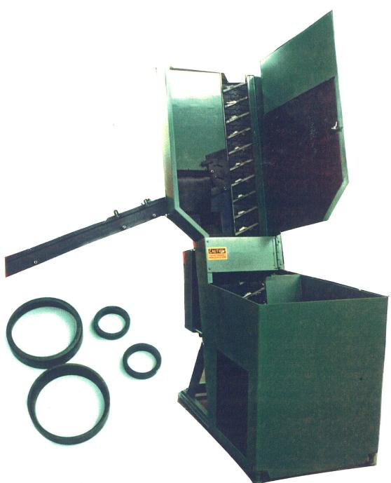
FEED FROM A RANDOM LOADED FLOOR MOUNTED HOPPER, VALVE SEAT INSERTS 1.00 TO 2.25" DIA. X .20 TO .50 THICK. THE SEATS WILL BE ORIENTED DIAMETER TO DIAMETER IN A SINGLE STREAM AND FED TO A HEIGHT OF 42" ABOVE THE FLOOR AT A RATE OF 200 PER. MIN. TO A FACE GRINDER. 7 1/2" WIDE ELEVATOR, 6 CU. FT. HOPPER. DWG. P 9179
