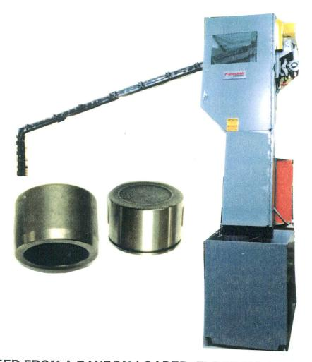
FEED FROM A RANDOM LOADED, FLOOR MOUNTED HOPPER, UNIVERSAL JOINT CUPS, 1.62 TO 2.36" DIA. X 1.12 TO 1.62" LG. THE CUPS WILL BE ORIENTED OPEN SIDE OUT THEN FED DIAMETER TO DIAMETER IN A VERTICAL STREAM TO A BRYANT GRINDER AT 52" ABOVE THE FLOOR AT A RATE OF 500 PER. HOUR. 7 1/2" WIDE ELEVATOR BELT, 6 CU. FT. HOPPER DWG. PD 9053
