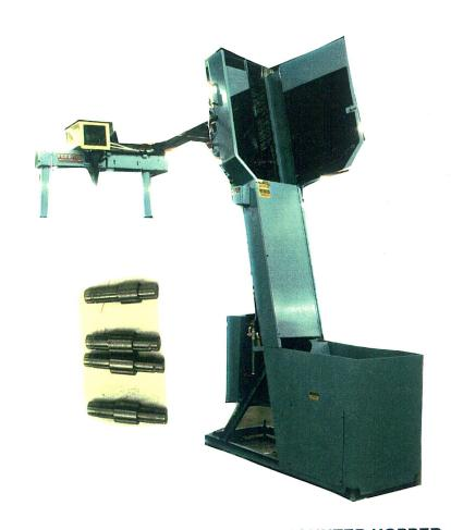
FEED FROM A RANDOM LOADED FLOOR MOUNTED HOPPER, PINION SHAFTS OF VARIOUS SIZES, THE SHAFTS WILL FIRST BE ORIENTED END TO END THEN FED TO A CONVEYOR THEN ORIENTED LONG END OF EACH SHAFT DOWN TO A VERTICAL CHUTE AT 88" ABOVE THE FLOOR AT A RATE OF 600 PER. HOUR.
