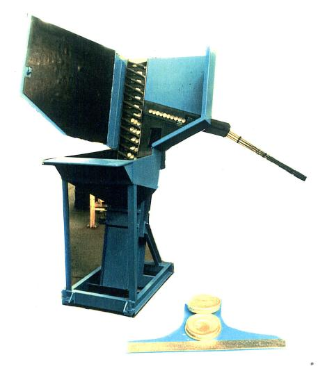
FEED FROM A RANDOM LOADED FLOOR MOUNTED HOPPER VALVE LIFTER FOOT CASTINGS. THE CASTINGS WILL BE FACE ORIENTED THEN FED ROLLING DIA. TO DIA. THRU A 90 DEGREE TWISTED CHUTE AND DELIVERED IN AN AXIS HORIZONTAL TO A HEIGHT OF 66" ABOVE THE FLOOR AT A RATE OF 50 PARTS PER. MIN. TO MACHINE CELL. 7 1/2" WIDE ELEVATOR BELT, 3 CU. FT. HOPPER. DWG. P 7799 R
