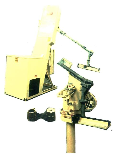
FEED FROM A RANDOM LOADED FLOOR MOUNTED HOPPER, SOCKET SHELLS OF VARIOUS SIZES. THE SOCKETS WILL FIRST BE ORIENTED END TO END THEN FED AND ORIENTED WITH THE AXIS VERTICAL AND THE HEX HEAD DOWN INTO A VERTICAL STACK TO A TRANSFER DEVICE ANDVANCING THE SOCKETS HORIZONTALLY DIA. TO DIA. AT A HEIGHT OF 42" ABOVE THE FLOOR AT A RATE OF 450 TO 500 PER. HOUR. 7 1/2" WIDE ELEVATOR BELT, 15 CU. FT. HOPPER. DWG. P7707 R 3
